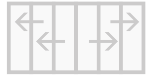
Centre Vent Stacking
